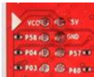
Figure 3. Pin-1 Marking on the CC3200MOD LaunchPad (White Triangle)
